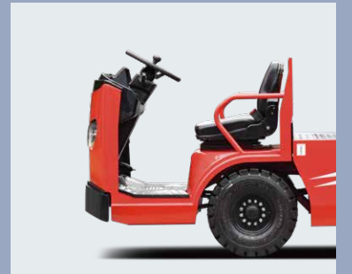
Full suspension operating platform, vibration is reduced, noise is isolated (1.5-5t)
